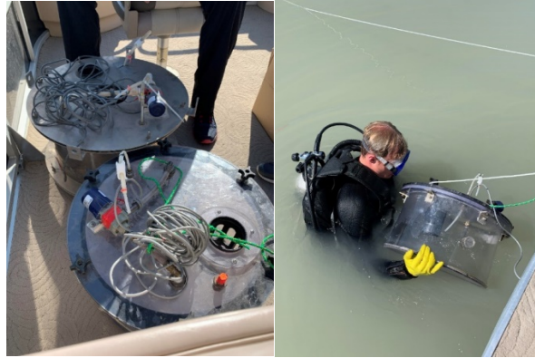
Figure 11. SOD chambers and installation in the field.
